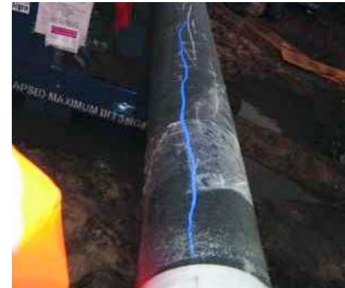
(a) K_0 < 1 Vertical fracture
